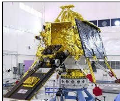
Fig. 2: Pragyan mounted on the ramp of Vikram Lander
